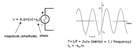
The phase determines when the sinusoid starts. It can be understood as a delay (t<sub>0</sub>) and its value can be either positive or negative.
