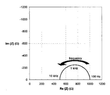
The imaginary part (with negative sign) of the impedance is plotted versus the real part of the impedance for each frequency. This representation is particularly used in electrochemistry and has been adopted by many researchers in the bioimpedance field. Its main advantage is that each dispersion is easily identified because it is displayed as an arc.
