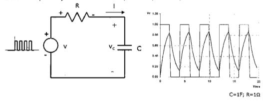
At the beginning the capacitance is discharged (Q=0 Coulombs) and, consequently, the voltage difference between its terminals is 0 V. The first input voltage pulse (plotted in red) causes some current to flow trough the resistance and starts to charge the capacitance. However, since the capacitance increases its voltage (plotted in blue), the current decreases and the voltage evolution is flattened.
