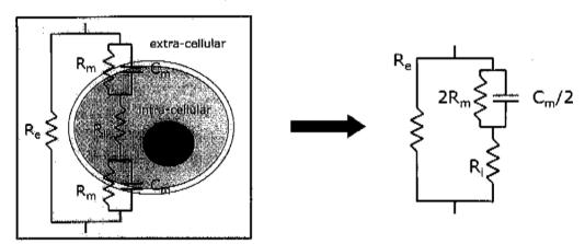
The circuit on the right is equivalent to the left model after performing some simplifications (resistances in series and capacitances in parallel). The same simplifications can be applied to reduce a tissue composed by many cells to a single cell equivalent circuit.
