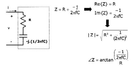
For R = 1 k $\Omega$  and C = 100 nF (10<sup>-9</sup> F) the following graphs are obtained:
