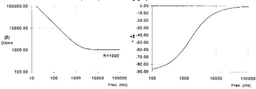
These graphs are the **Bode plots** of the impedance. On the left, the magnitude, or modulus, of the impedance is displayed for each frequency (f). Both axes, horizontal and vertical, are expressed in logarithm base 10. The graph on the right shows the phase value for each frequency. In this case, only the frequency is expressed in the logarithm form.
