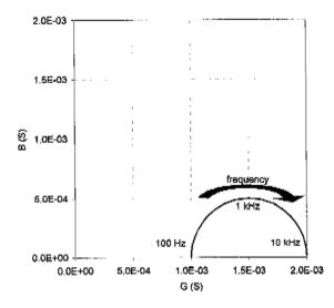
The scaling factor (K) is  $(\pi \times 1 \text{ cm}^2)/(2 \text{ cm}) = 1.57 \text{ cm}$ . Then, the conductivity  $(\sigma = G/K)$  and the relative permittivity  $(\epsilon_i = \epsilon/\epsilon_0, \ \epsilon_0 = 8.8 \times 10^{-14} \text{ F/cm}; \ \epsilon = B/(\omega K) = B/(2\pi f K)$ ) can be obtained from the conductance (G) and susceptance (B) values:
