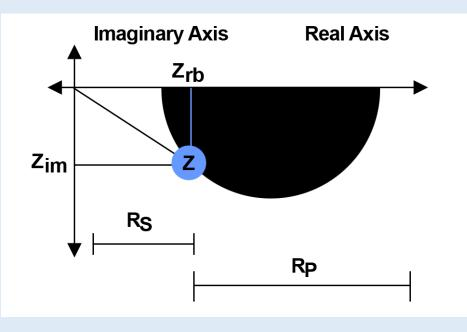
The impedance locus of the circuit shown in slope above forms a circular arc in the IV quadrant of the coordinate system.  $R_S$  and  $R_P$  can be derived from the intersections with the abscissa of the extrapolated bio-impedance curve.
